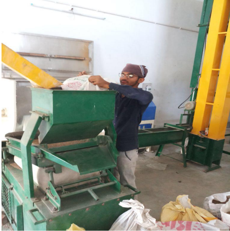
Cleaning and destoning
